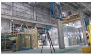
▲Fans and a dust counter (center) used to measure dust particles. Sources of dust are covered by sheets.
