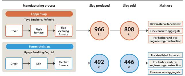
Copper slag is a by-product produced during smelting at the Toyo Smelter & Refinery, which manufactures electrolytic copper. The main use for copper slag (70% of the total volume) is cement production for Japan and overseas. With an iron content of about 40%, copper slag is widely used as a source of iron for cement.
