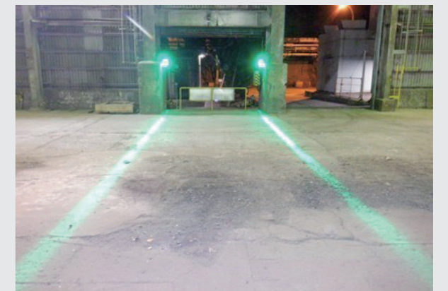
Demarcation of walkway boundaries using light
