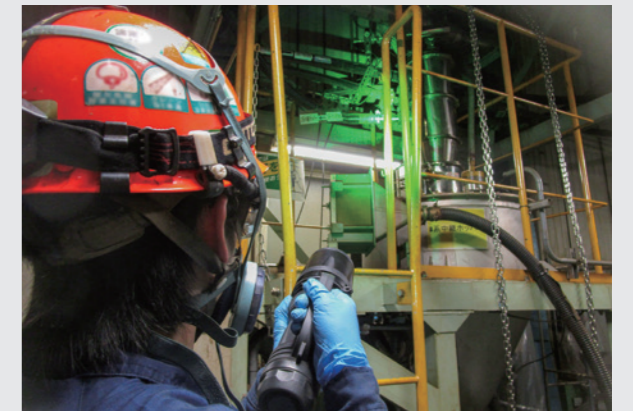
Identification of dust sources using a special-purpose light
