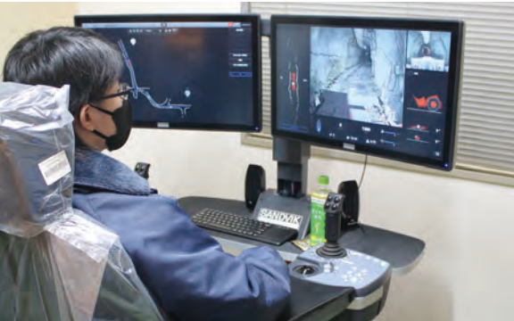
Remote operation of heavy equipment at the Hishikari Mine from above ground
