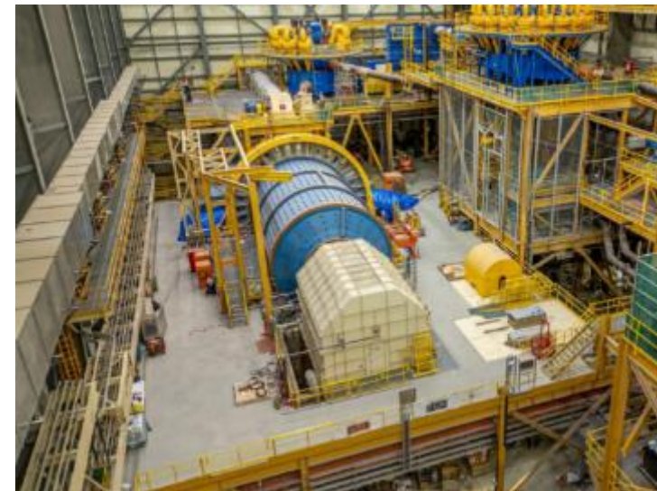
Ball mill inside the ore processing plant (January 2024)
