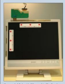
Copper-clad Polymide Film used in Flat Panel LCD TV Copper-clad Polymide Film is used in the places indicated by the arrows
