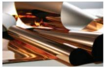
Copper-clad Polyimide Film A board material consisting of polyimide film on which copper has been vapor-deposited, this is mainly used in the COF boards that package the ICs that drive LCDs.
