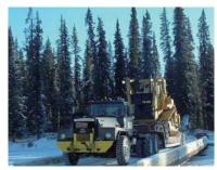
Heavy machinery transport via winter road Cold temperatures were needed to ensure sufficiently thick ice to enable transportation of the heaviest equipment
